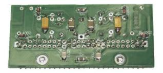
In our High-End amplifiers we separated the VS-module power lines from the CS-stage power lines. Due to this we are able to provide regulated supply voltages for this input stage VS-module of our High-End amps. This will bring the effects as described above.
